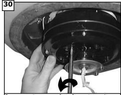
Remove motor screws from fan motor and save.
